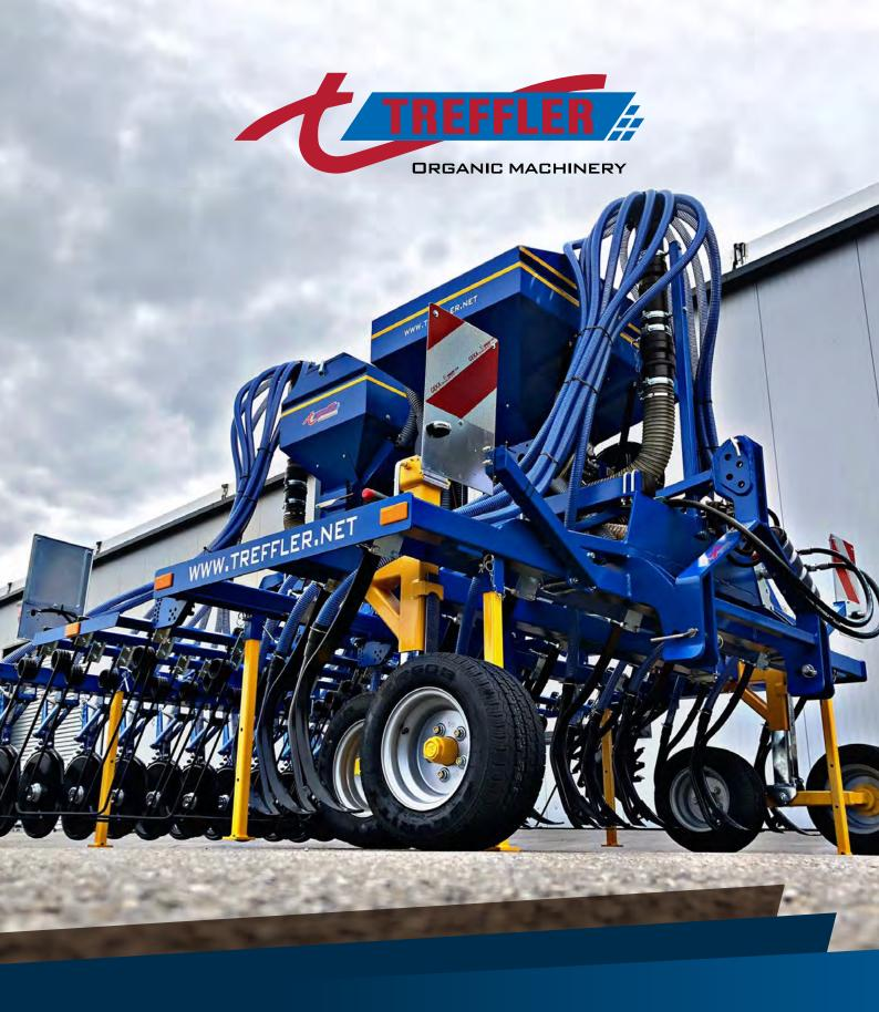
TKM combined sowing machine 3.0 m (10 ft) working width
