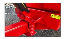
Redrock Dump Trailer bodies are constructed with vertical supports integrated into the chassis to give the maximum possible support and strength for heavy loads. All Dump Trailers have a sprung drawbar for increased driver comfort and to reduce stress on the tractor hitch.
