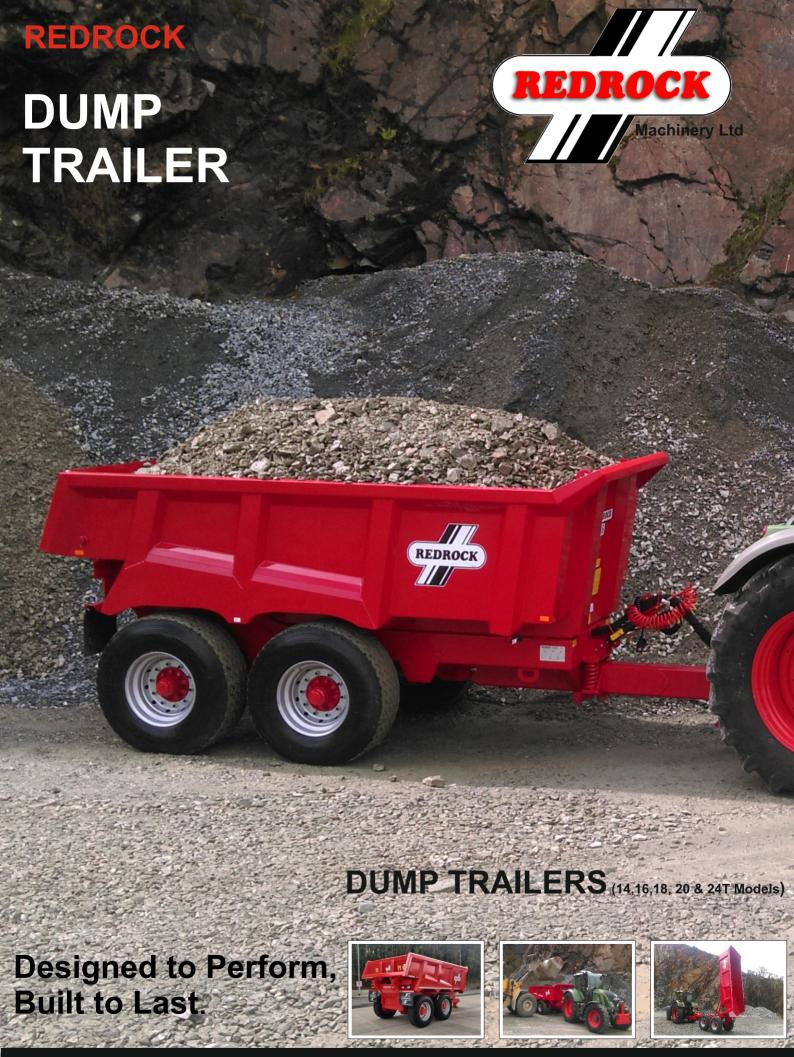
For the toughest jobs, you need the toughest trailers. Redrock's Dump Trailers feature an innovative fold down door configuration, to make tipping easier and safer. 14 & 16 ton trailers come with 8mm floor and 6mm sides and 18 - 25 ton trailers come with 10mm floors and 8mm sides. Hardox steel option is available on request.
